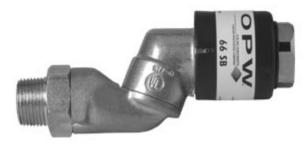
The OPW 66SB Swivel Breakaway is intended for easy installation at the nozzle inlet. The compact, lightweight design incorporates a 360° swivel rotation at both the male end and middle joint, with a simple and easily reconnectable breakaway on the opposite end.
