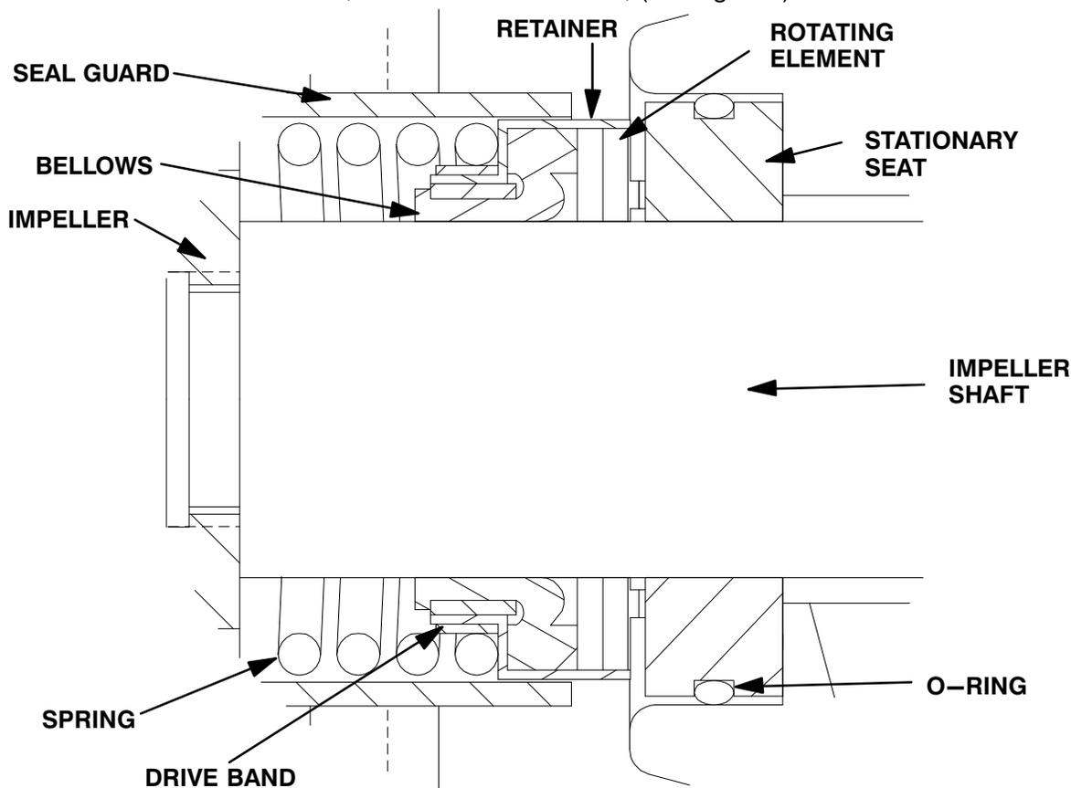
Figure 4. 25271-851 Seal Assembly
