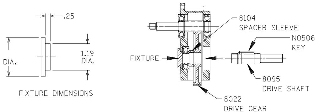
**Figure 5. Fixture Dimensions, Drive Gear And Shaft Installation**
