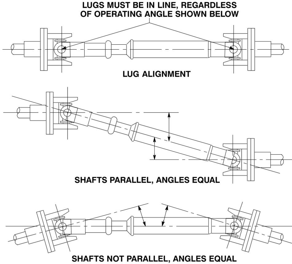
**Figure 3. Proper Installation And Alignment of Universal Assembly**
