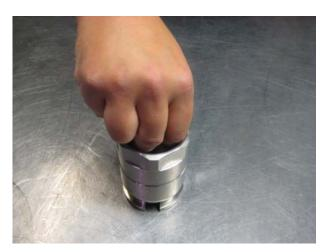
Press down the spindle steering and turn, to fix it in its position.
