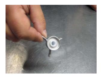
Replace the Teflon® bushing (pos.5) in the spindle steering with a new one.
