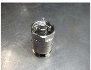
Replace the spring (pos.7), springcap (pos.6) and the spindle steering (pos.4).
