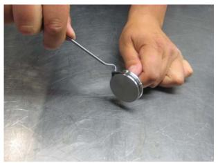
Replace the O-ring (pos.3) on the piston with a new greased O-ring.
