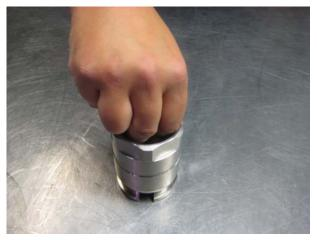
Press down the spindle steering and turn it free.
