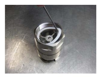
Remove the flat sealing NPT-thread doesn't have a flat sealing.
