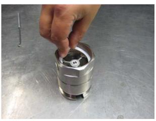
Assemble a new flat sealing (pos.12). NPT-thread does not have a flat sealing.
