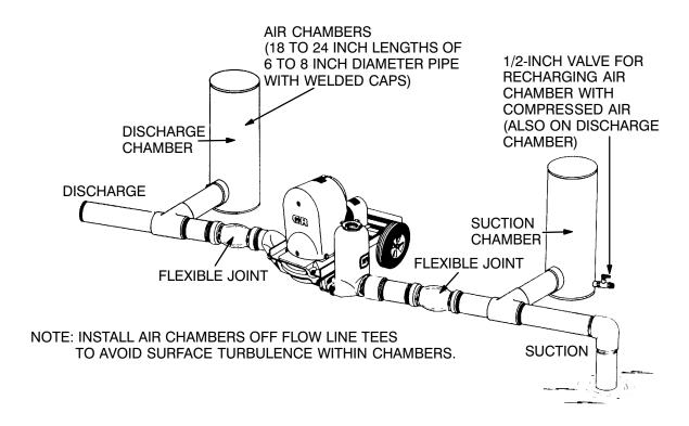
Figure 2. Fixed Piping Installation
