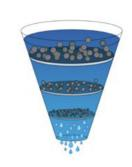
High efficiency (ß 200) mechanical filtration of particulate by means of an incremental filter specifically developed for DEF.
