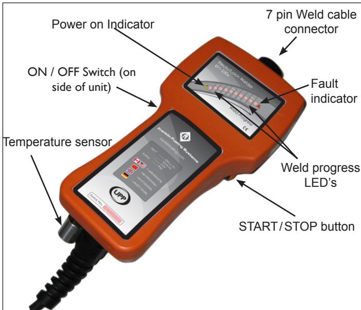
The EF1 takes the ambient temperature into account when calculating the energy required to weld correctly. It must therefore be allowed to reach ambient temperature before use and must be at the same temperature as the fitting to be welded. The temperature sensor is located adjacent to the power cable entry gland.
