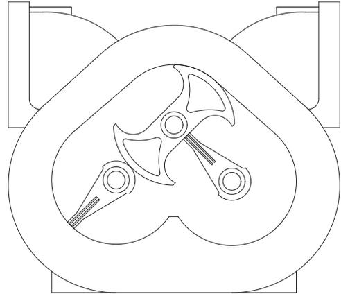
The rotors in the meter are designed to operate at close tolerances to one another and the wall of the fluid chamber. There are slight clearances between the rotors and the chamber wall. Because of this, it is important that the meter be properly applied for the flow rate and operating pressure of the system.
