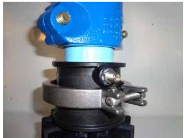
**Figure 4: Clamp in Position**
