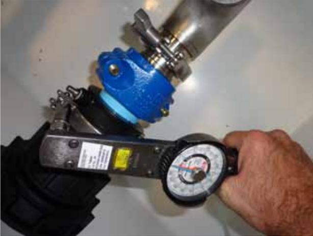
**Figure 5: Tighten Nut**
