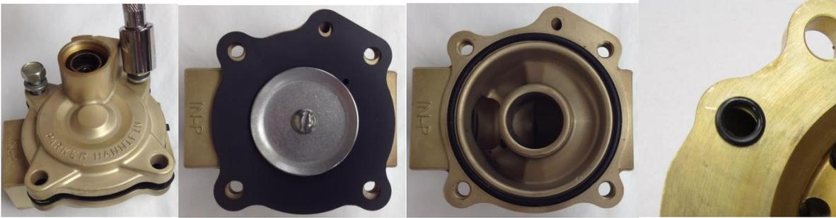
7. Remove the diaphragm spring, diaphragm, the large body O-ring, and the small pilot port O-ring. Discard all.
