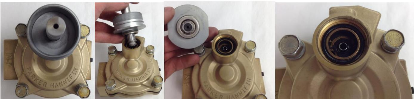
4. Remove lower plunger & spring assembly, upper plunger, upper plunger seal, upper spring, and flange O-ring.
