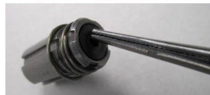
5. Discard upper plunger seal, upper spring (if desired), and flange O-ring. Remove and discard the lower plunger seal.
