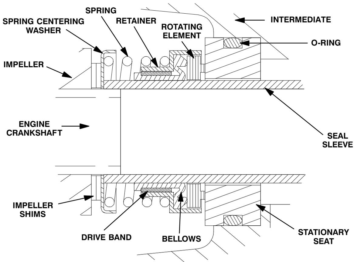
Figure 4. Seal Assembly
