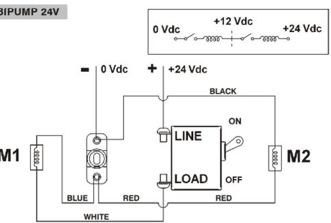
In the event of a 24V connection without switch, connect the white cable directly to the positive pole (+).
