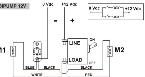
In the event of a 12V connection without switch, connect the white and red cables directly to the positive pole (+).
