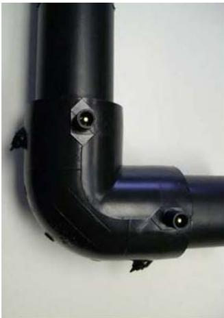
UPP pipe is very similar to NUPI. It has a black or green polyethylene secondary and a black primary. UPP uses black electro fusion ends and couplers.
