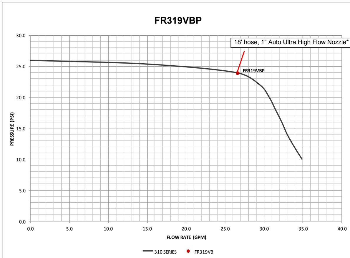
*Changes in temperatures, fluid viscosity, and system accessories may shift the performance curves.*
