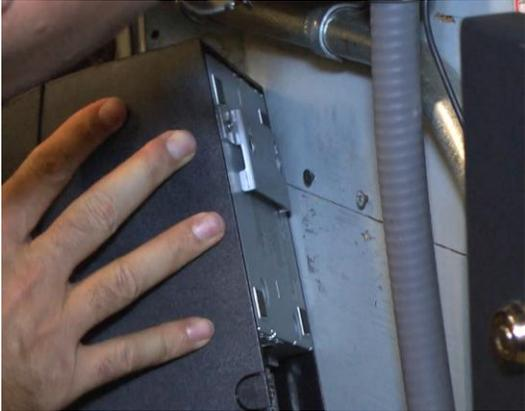
Figure 3-3 Install External Thermal Printer
