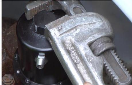
Figure 11-4 Tighten Sensor
