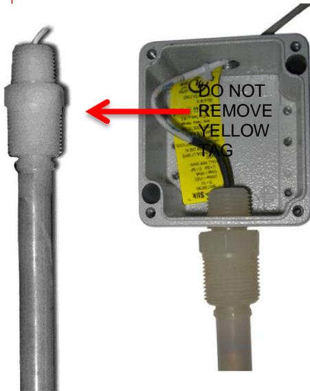
Figure 10-1 Model 7100V Flex Probe
