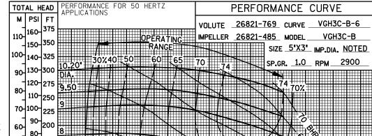
50 HERTZ PERFORMANCE **BASED ON** WATER **TRIMMED IMPELLER**
