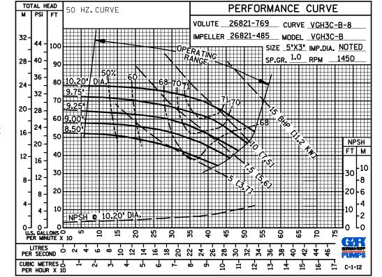
**50 HERTZ PERFORMANCE BASED ON** WATER **TRIMMED IMPELLER**
