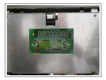
2 After the required can size appears on the display, remove the nozzle and switch on the pump handle. This selects the can size for calibration.
