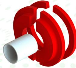
The FLX Series is used for internal, one-sided repairs to eliminate continuous leak points caused by degraded flexible entry boots in singlewall sumps. FLX fitting kits are universal for round or flat sump walls and the split design doesn't require excavation or disconnecting pipe. Models available for all common flex pipe and semi-rigid piping. Quality FRP construction provides long term compliance solutions.
