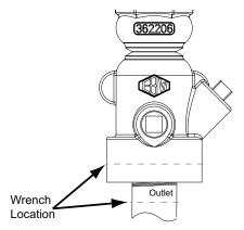
**NOTE:** The dispenser pipe can be connected to the top or side inlet port. If you wish to use the side inlet port, remove the 1" plug, apply the sealing compound to the threads, and install the plug into the top inlet port.
