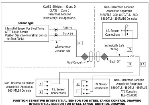
**CSTP LIQUID SWITCH CONTROL DRAWING**
