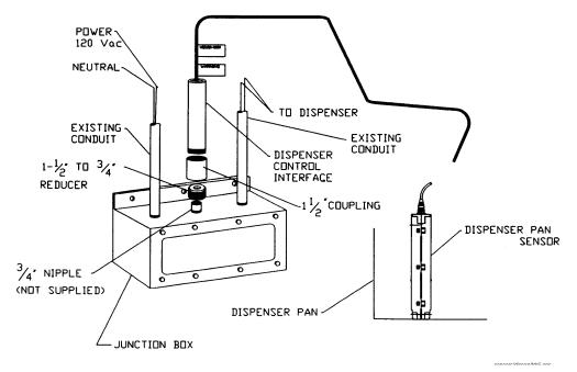
Figure 1. Typical Dispenser Control Interface Installation
