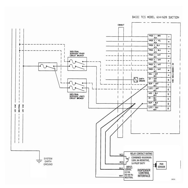
**Figure 6.** Typical Installation Wiring Diagram for Dispenser Control Interface to a Tokheim Basic TCS Model 614/628 Dispenser
