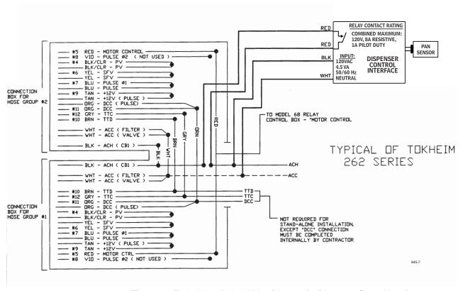
**Figure 7.** Typical Installation Wiring Diagram for Dispenser Control Interface to a Tokheim 262 Series Dispenser
