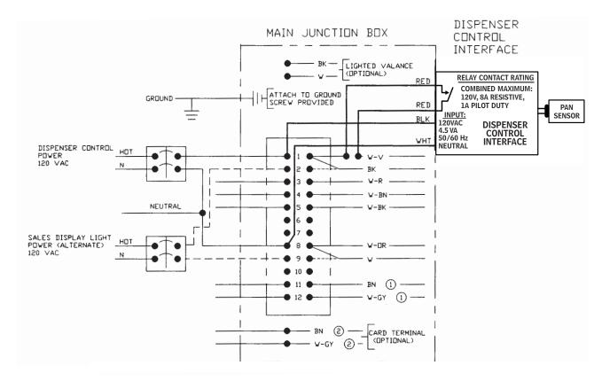
**Figure 4.** Typical Installation Wiring Diagram for Dispenser Control Interface to a Dresser-Wayne Dispenser (120 VAC)
