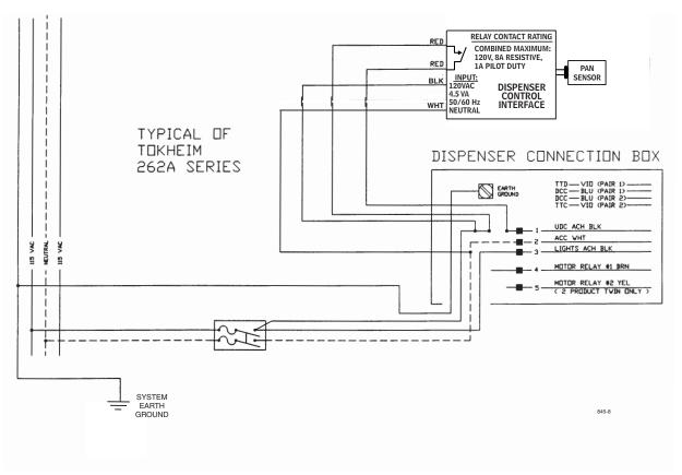
**Figure 8.** Typical Installation Wiring Diagram for Dispenser Control Interface to a Tokheim 262A Series Dispenser
