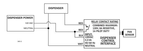
Figure 3. Typical Dispenser Control Interface Wiring Diagram
