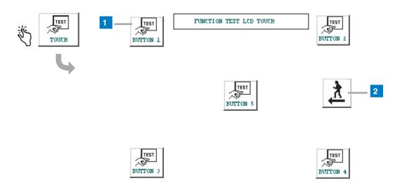
This screen displays 5 test buttons (e.g., item 1) around the display. Touch one of these buttons and a message appears showing that button's corresponding x/y coordinates and a look up list with the correct coordinates for all 5 buttons).
