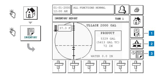
To view the inventory report for a tank, touch the inventory report button for the desired tank at the bottom of the screen. To view the Shift Inventory report for the selected tank, touch the Shift Inventory button (item 1 in the screen above). To view the stick height (if enabled) for the selected tank, touch the Delta Stick button (item 2 in the screen above). To view the Inventory Log report for the selected tank, touch the Inventory Log Report button (item 3 in the screen above).
