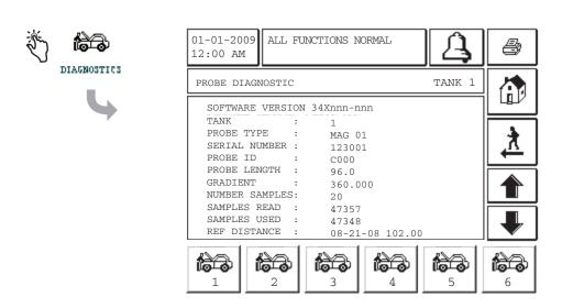
Touch the down arrow to view available probe temperature data. To view another tank's probe diagnostics, touch the desired tank's Diagnostic button at the bottom of the screen.
