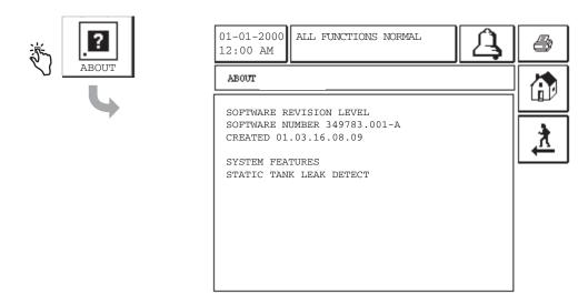
This screen lists information about the TLS2 Console's installed software and features:
