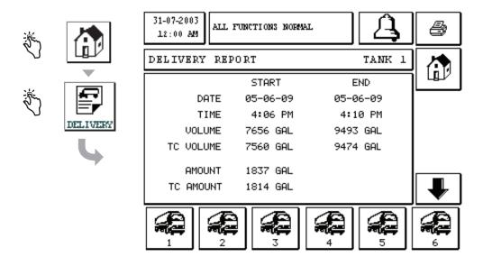
Touch the Tanker button at the bottom of the screen to view a delivery for that tank.
